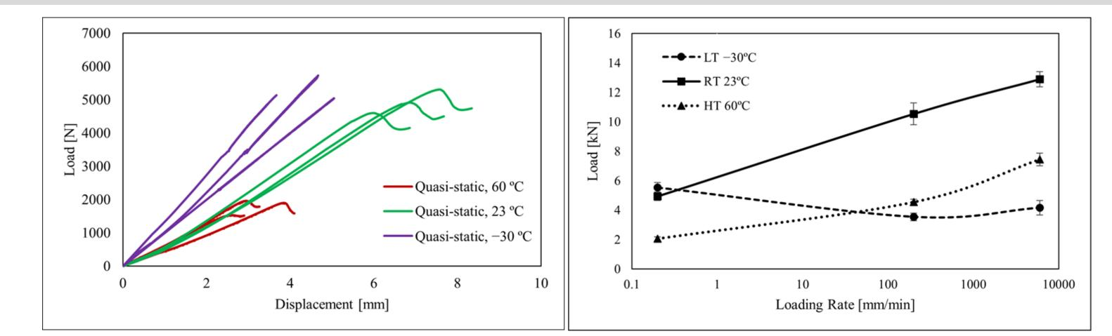
Figure 5 – Load-displacement of the machine for test submitted to quasi-static conditions for a mixed mode apparatus set up at 45°.
