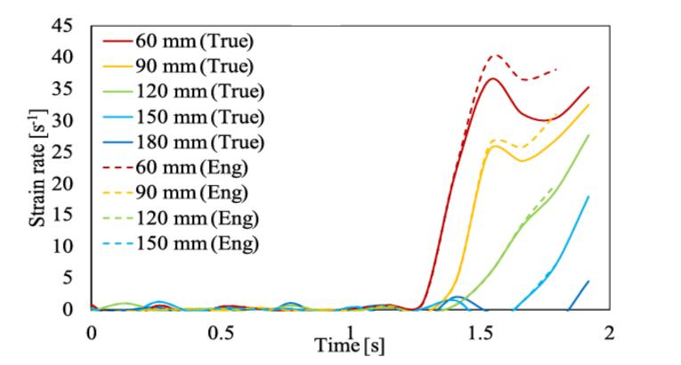
Figure 4 – True and engineering strain rates as function of time for different distances of the DCB edge (200 mm/min, -30 °C)
